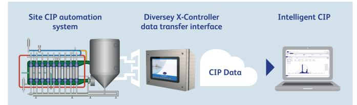
Diversey Intelligent CIP uses the power of cloud-computing to collate and process your CIP data, giving you immediate insight into the performance of each cleaning run.
